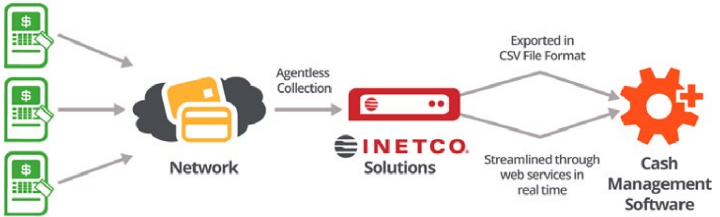
DIAGRAM 1 - The path of the ATM transaction data, showcasing the integral role of INETCO solutions in monitoring and forwarding data to cash management software. Data can be either exported in csv format or streamed in real time through web services.
